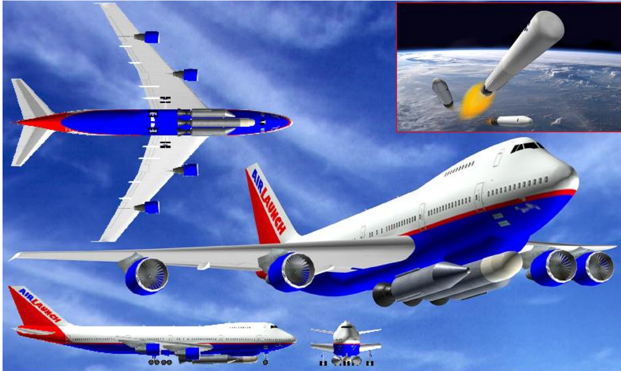
Fig. 7 747 Carrier Aircraft with 3 barrel, 3-stage-to-orbit Launch Vehicle
