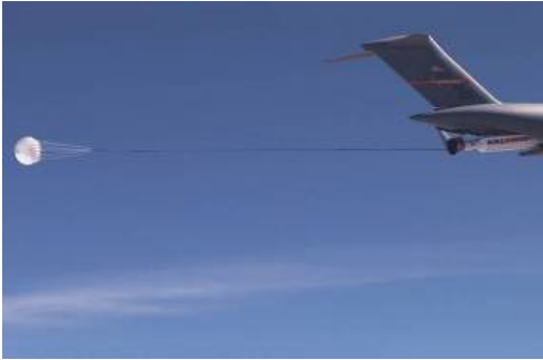
C-17 Drop Test of Simulated QuickReach™ Small Launch Vehicle Photos Taken from F-16 Chase Plane
