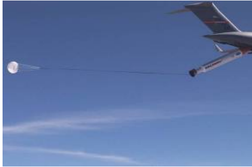
C-17 Drop Test of Simulated QuickReach™ Small Launch Vehicle Photos Taken from F-16 Chase Plane
