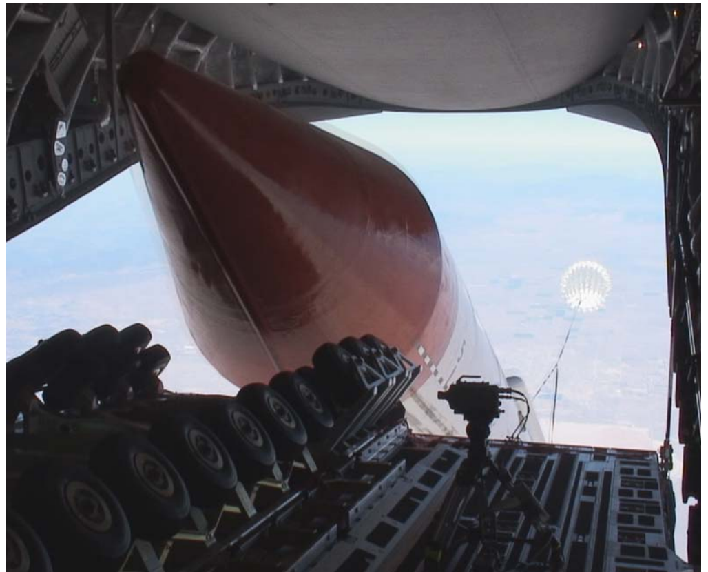
AirLaunch Drop Test Set Record for Heaviest Single Object (65,000 lbs) Dropped from a C-17
