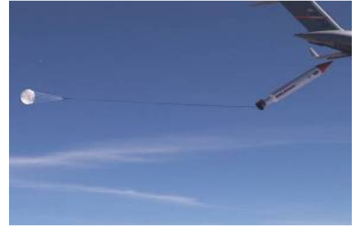
C-17 Drop Test of Simulated QuickReach™ Small Launch Vehicle Photos Taken from F-16 Chase Plane
