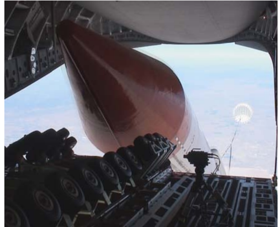
AirLaunch drop test sets record for heaviest single object dropped from a C-17, June 14, 2006
