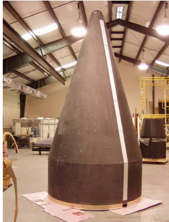
QuickReach™ payload fairing assembled as part of Milestone 3
