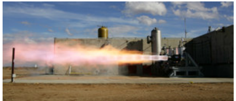
Stage 2 engine hot fire test program begun
