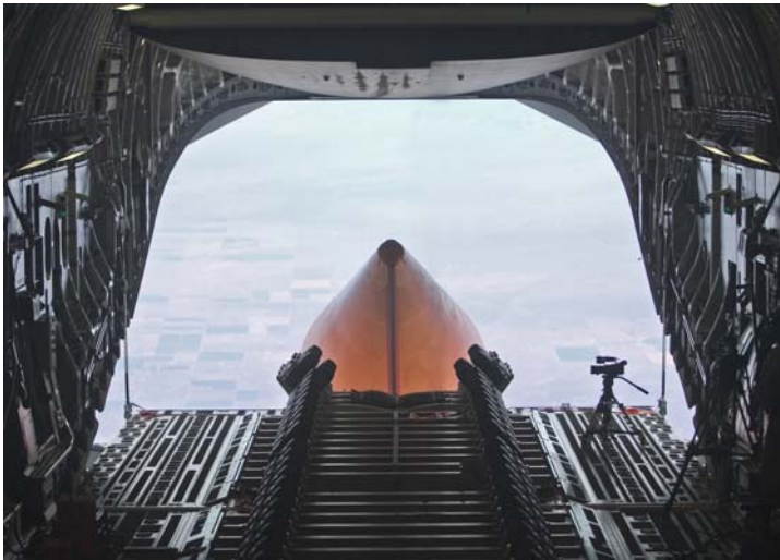
QuickReach™ 72,000 lb Test Article Released from the C-17 – A New Record for the Heaviest Single Object Ever Dropped from the Aircraft
